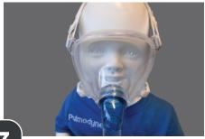
After adjusting the straps, make sure the mask hasn't moved around. Check to make sure the cushion is above the eyebrow and below the lower lip.
